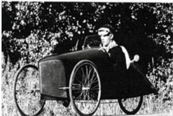
several years. As the first kinneris were heavy made of timber and plywood, Sammalisto was using aluminium both in tubes and plates. His gears could both make the thing go fast and climb steep hills.
